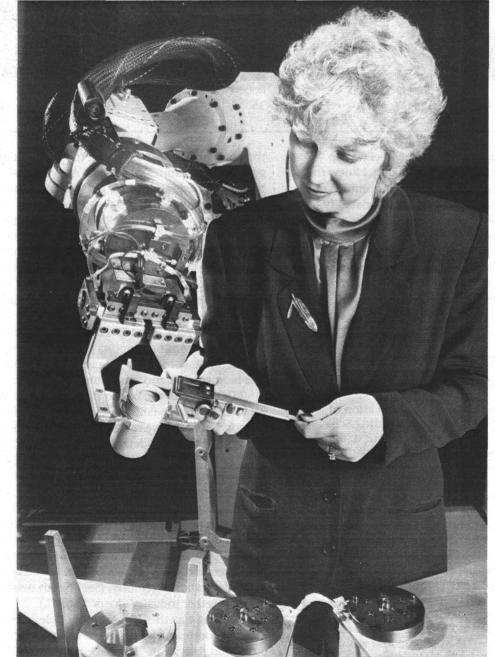
Carla Montoya (9671) measures a mockup of a nuclear weapon gas generator held by Sandia's Automated Gas Generator Disassembly System (AGGDS). The system is currently being installed for disassembly work at the Pantex Plant near Amarillo, Texas.
